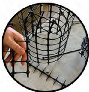
Tensar (outer shell held together with zip ties)
