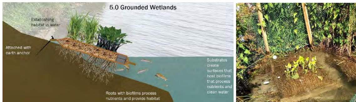
Figure 4.1: Pillow-like 5.0 wetland that moves with the water level
