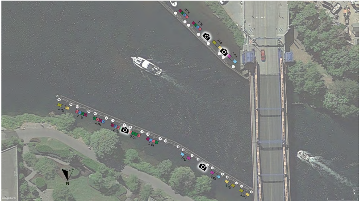
Figure 3.3.2: Shows the locations of the cameras deployed at Fremont. There were 4 cameras attached at the fender wall, 2 control and 2 at units. Another camera was attached to the Sonde and suspended to the bottom of the channel and also moved along the shorelines.
