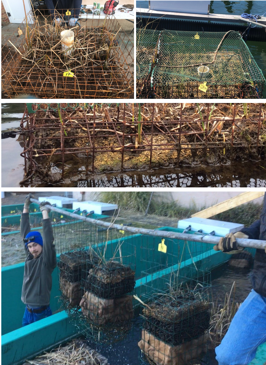
FIGURE 4. Photos of ABS piping in the wetland biofilters (upper left); goose netting on wetland biofilter (upper right); degrading substrate (middle); puck (1' x 1' wetland biofilters) showing the material layers.
