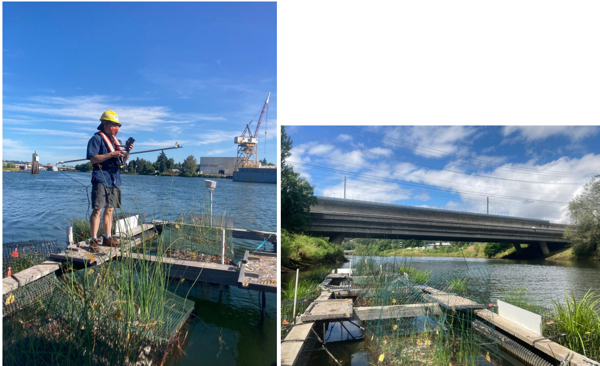
Figure 1.1 Left, water quality lead, George, preparing flow meter to monitor water velocity at Waste Management site Biobarge B. Right shows the Biobarges at the Tukwila Site, (July 19 2020).
