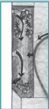
bio-swale treating road & walkway run-off
