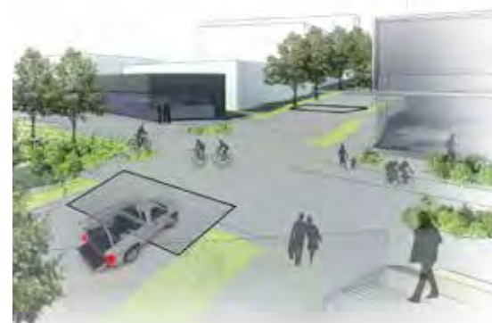
Traffic table at Brooklyn Ave and Burke Gilman St from Outreach Center elevated park space
