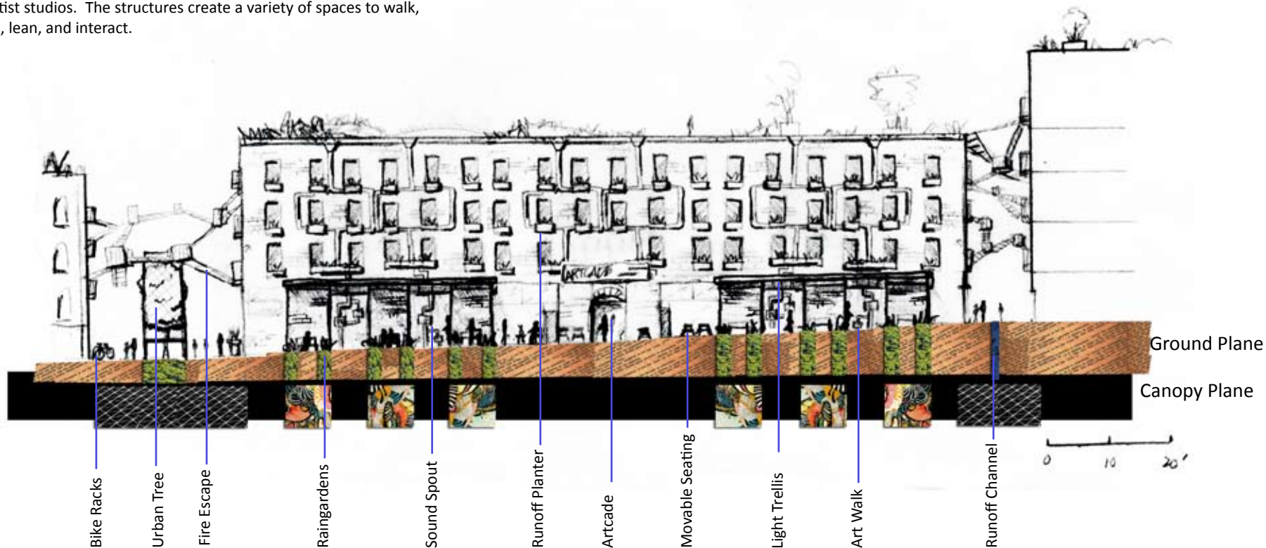
Section BB looking North. The ground, wall, and canopy planes create a rhythm for the senses. The experience is unified by light, water, glass, and steel. The Soundspouts, during, storms produce an audio experience of splashing and pulsing. The Raingardens capture runoff from the Art Walks Light Trellis and the surrounding hardscape. Steel fire escapes play off historical reference and frame views. The Arcade provides studio space. The greenroof is a private retreat for residents of the north and south buildings.
