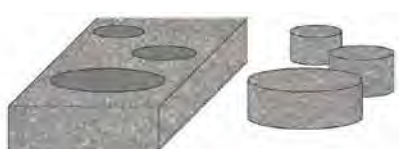
Hollow cores are created in salvaged concrete blocks from the viaduct
