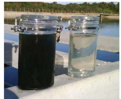
Left canister displays water from influent of the treatment lagoons and right canister displays water taken from effluent. The decrease in TSS is readily visible.
