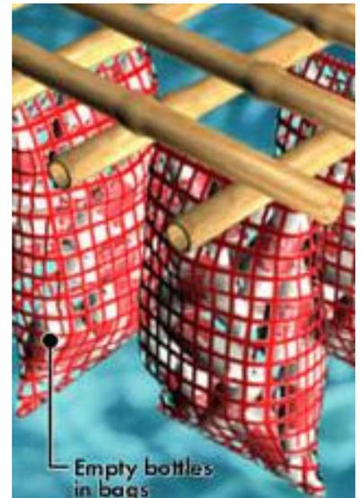
Plastic bottles in mesh bags are connected to a bamboo frame, supporting the island and allowing it to float.
