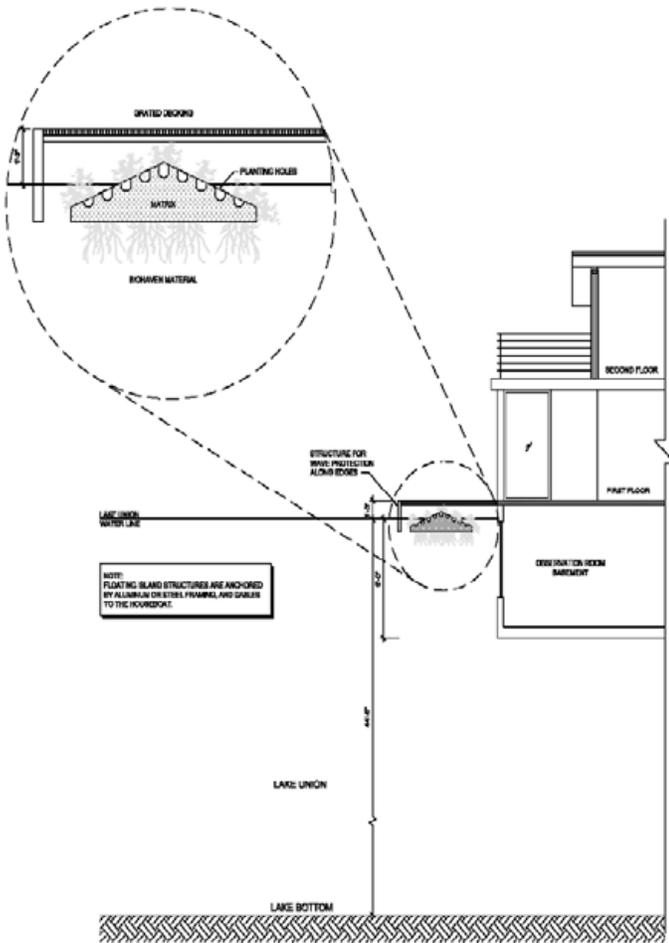
NOTE: FLOATING ISLAND STRUCTURES ARE ANCHORED BY ALUMINUM DRIFTLINK PIVOTALS AND CABLES TO THE ROVDECKPORT.
