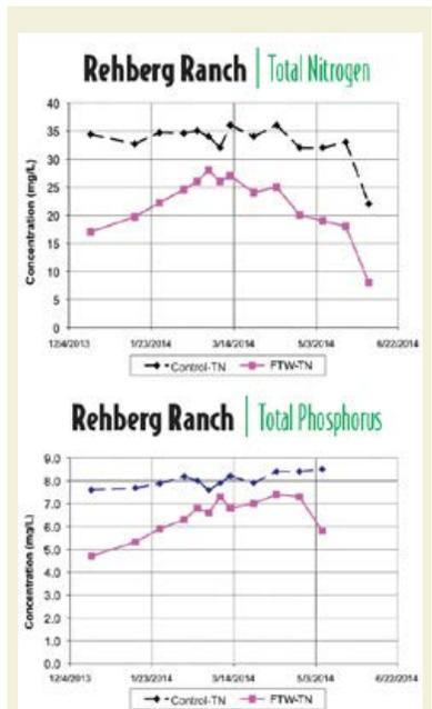
The Rehberg Floating Treatment Wetland (FTW) has proven effective at removing nitrogen and phosphorus.
