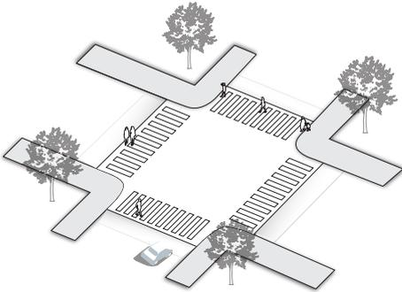
**Vertical Elements** (Including Raised Intersections (above), Speed Tables, Speed Humps, etc.)
