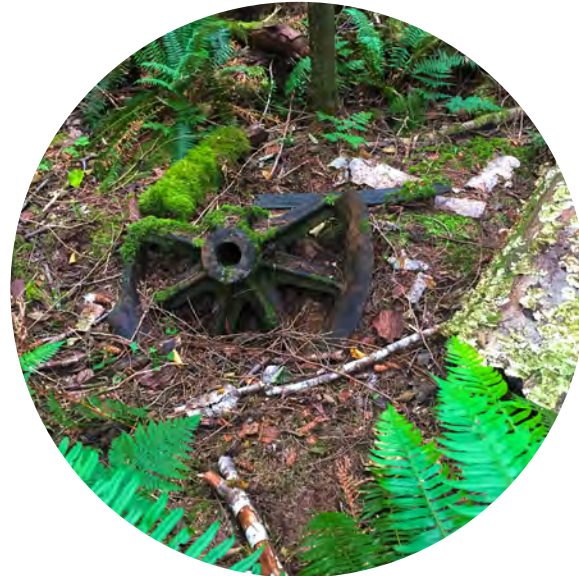
2. A concave wheel was used on wooded rail tracks that hauled recently cut logs up and down the mountain.
